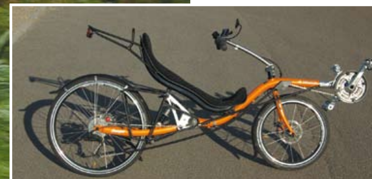
ABOVE: The Fuego can be adjusted without tools through quite a range of ride heights and seat angles.
