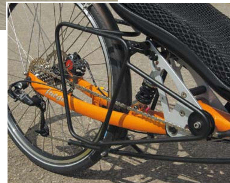
BELOW: Several tidy details to note here, including the curve of the carrier rack around that chain pulley, the solid low-rider pannier rack and the multi-position support for the rear shock.
